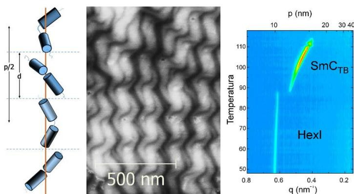
**Fig. 1** *left*: model of  $SmC_{TB}$  phase; *middle*: AFM image of HexI phase registered at room temperature, showing twisted filament morphology; *right*: temperature evolution of resonant X-ray diffraction pattern in the  $SmC_{TB}$  and HexI phases of homologue  $n = 7$ .
